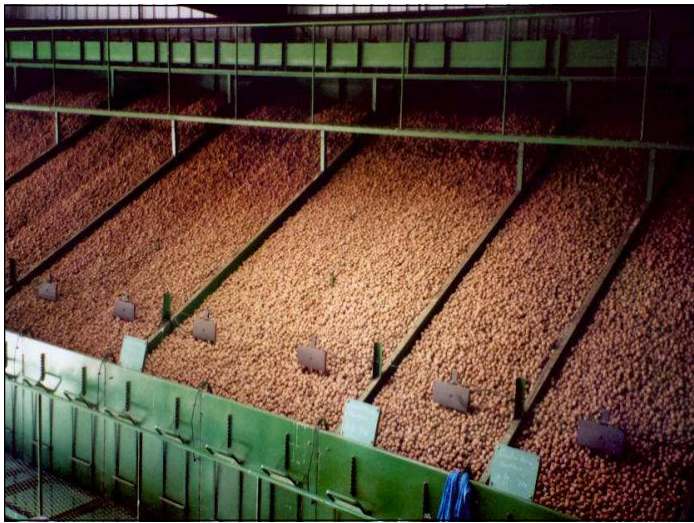
Above: In the drying chamber a portion of the warm air rising from the walnuts is recirculated back to the blower and mixed with the solar heated air. Left: Walnuts being dried with solar heat.
