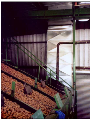
Typical multi bin walnut dryer. A duct from the roof distributes the solar heated air to the two air inlets for the blower.
