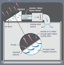
ing the night sky by as much as 10 C (18 F) below ambient. Using the HVAC economizer control strategy, the SolarDuct system allows outside air passing through it to radiate heat to the night sky which cools the air below ambient.
