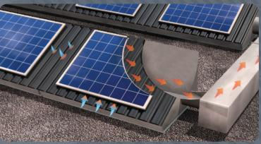
The SolarDuct® product can also be used for PV/thermal cogeneration systems. With a SolarDuct PV/T system, the all-metal SolarWall® absorber doubles as the PV-racking system and draws heat away from the PV modules. This heat energy is then ducted to the nearest rooftop air handling unit and then into the building's conventional HVAC system to offset the heating load. The removal of the PV heat cools the modules and enhances the electrical operating efficiency of the PV (up to 10%).
